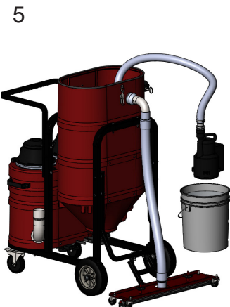
Place the pump in a 5 gallon bucket and run the clean water through the pump.
